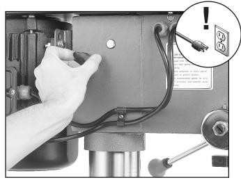
Figure 26. Loosening lock knob (both sides).
